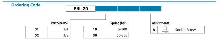
Ordering Code Example: PRL200230A - 3/8 BSP - 50-350 bar setting range, Socket screw adjustment.
